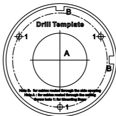
Figure 2-11 Drill Template of Junction Box
